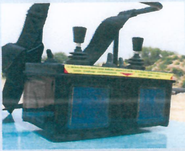
IR transmitter with solar panels
