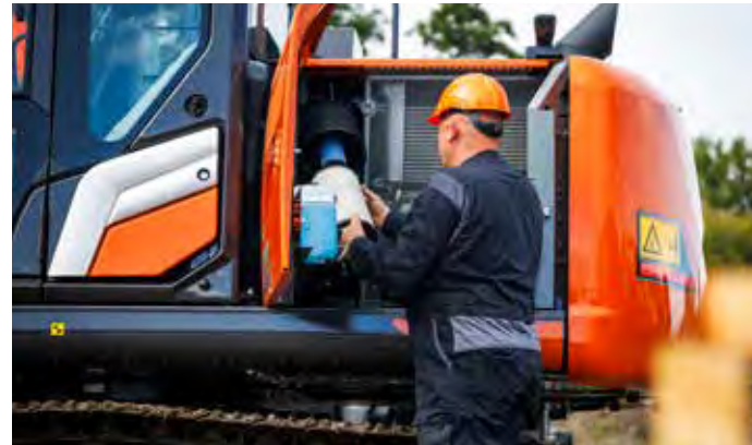
Access to filters has improved on the ZX135US-7B.
